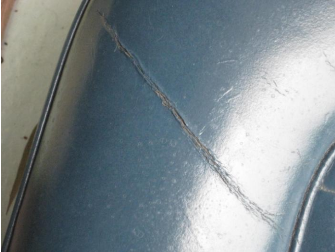
SMALL CRACKS DISAPPEAR AS THE LEATHER TAKES ON ITS ORIGINAL SHAPE – LARGER CRACKS LIKE THIS ONE NEED TO BE FILLED USING FLEXIBLE CRACK FILLER
